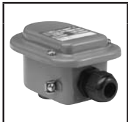
TYPE 03: Metal, epoxy coated / AISI 316 SS WP / WS: IEC 335 EM / WSEM: EN 60079-7/18 and EN 61241-1
