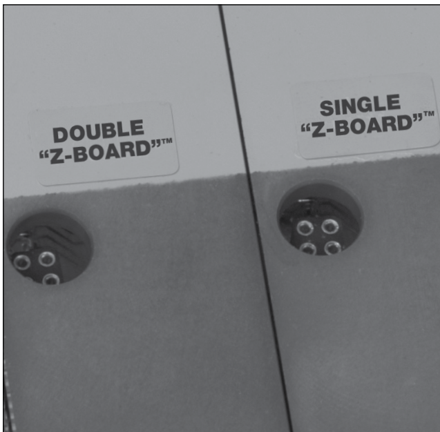
Label on manifold block indicates installed "Z-Board"™ type.
