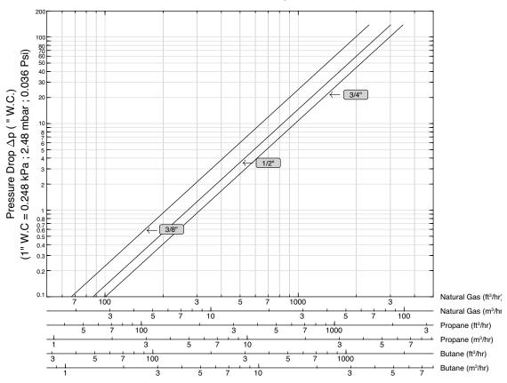
$\textbf{Note:} \ \ \text{Flow curves are based on the following standard conditions: 5 psi (0.3 bar) inlet pressure and 68°F (20°C) fluid temperature.}$
