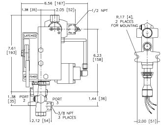
IMPORTANT: Mount with manual reset assembly vertical and upright.
