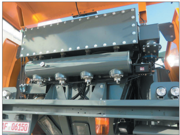
Custom Tank system solution with integrated two-stage pulse diaphragm valves 1 1/2". External control via pilot valve box.
